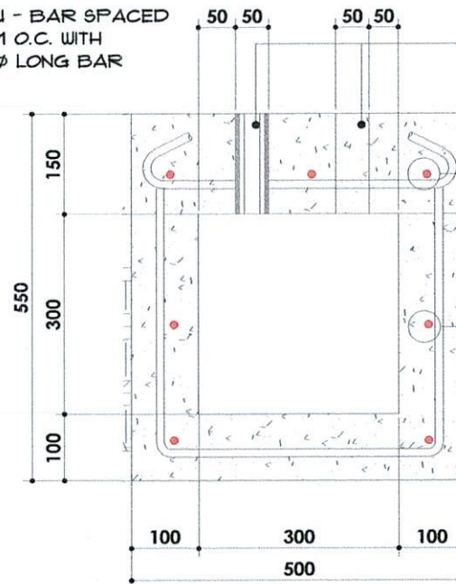
COVERED CANAL SECTION 2
